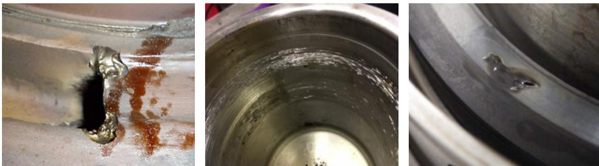
Figure 1. (a) Centrifugal pump wear. (b) Magnetic drive pump wear. (c) Mating ring wear & residue.
