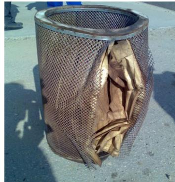
Figure 3. Examples of damaged strainers.
