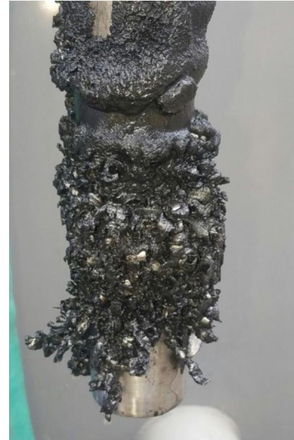
Contamination captured after 18 hours in a desalter water test.
