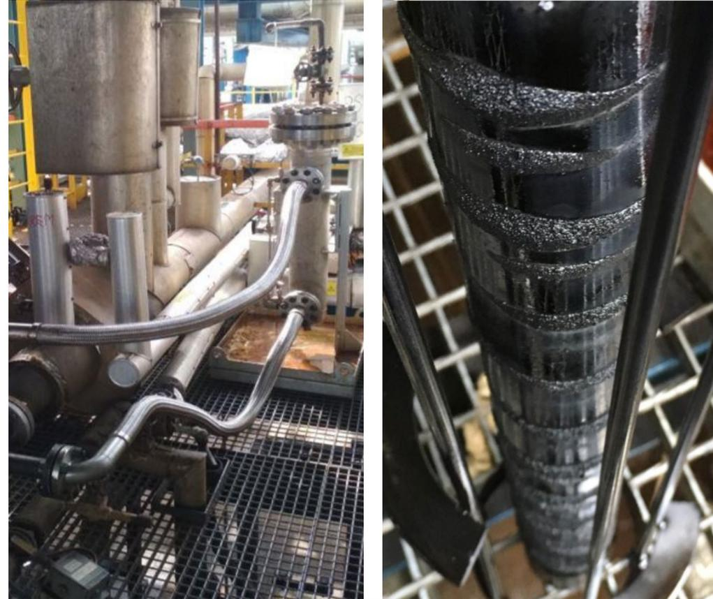
BPS magnetic separator installed in the HDS amine system during testing, as well as contamination captured after 2 weeks of testing.
