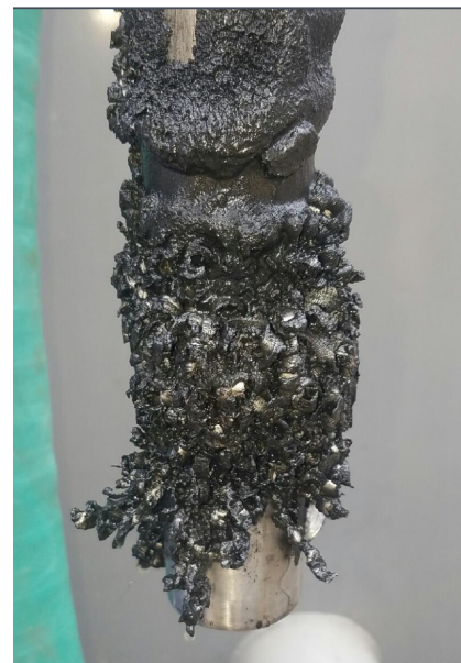
Black powder collected on the first magnetic separator element after 18 hours of operation.
